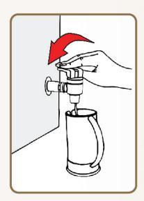
Push to lock for continuous flow. Return the lever to stop. If lever does not lock, rotate it 180° before dispensing.
